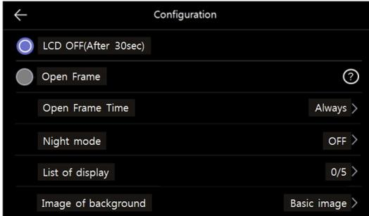
LCD OFF(After 30sec) : To set screen off function when entering standby mode
